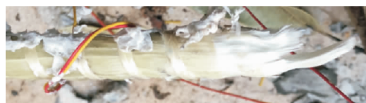
(c) 90^\circ 筋材折角断裂形态
